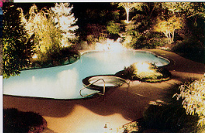
Low-voltage lighting transforms this backyard pool and spa area into a nighttime wonderland. By using low voltage, the designer was able to bring light close to the water's edge.
